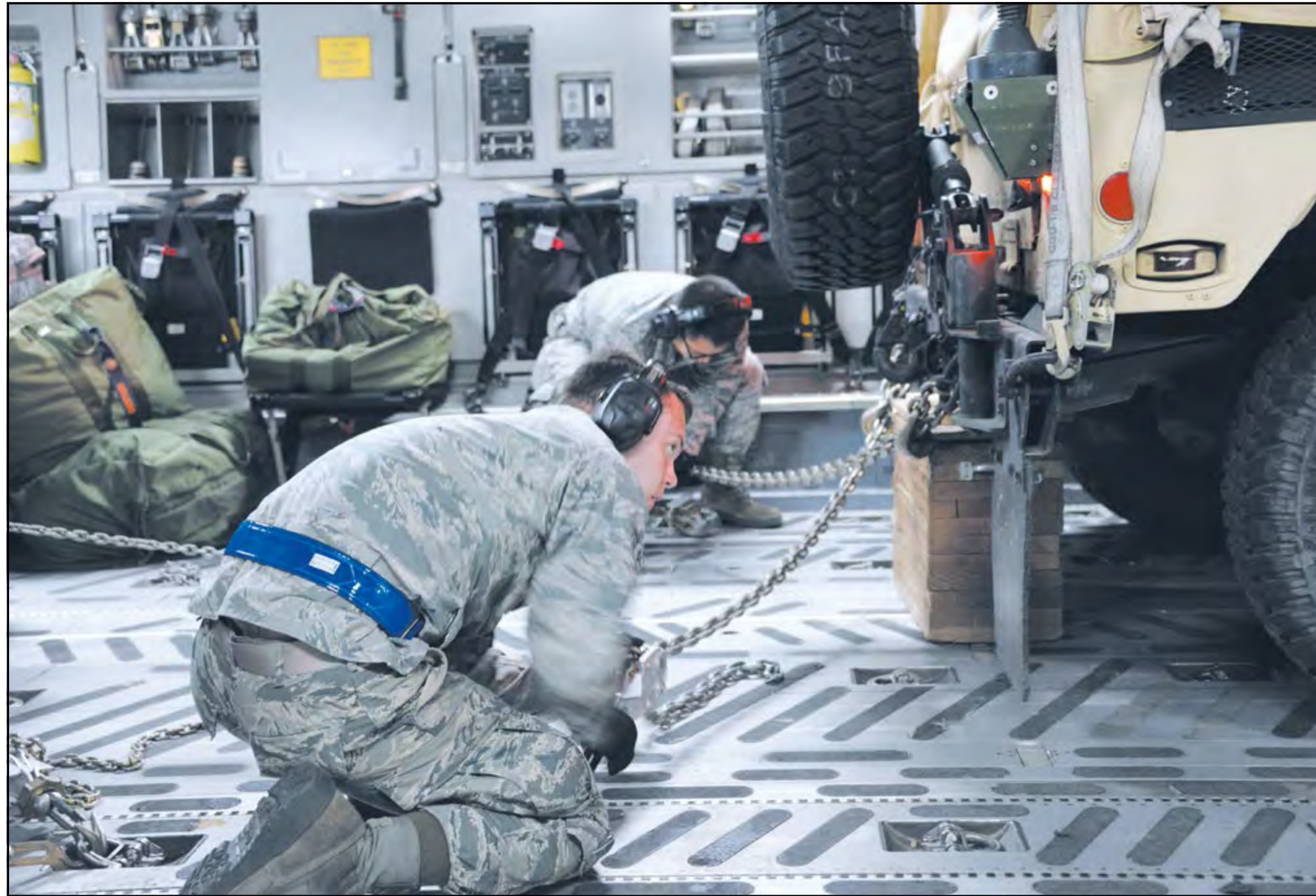
Members of the 60th Aerial Port Squadron at Travis Air Force Base, Calif., load a C-17 Globemaster III Sept. 7 with two all terrain vehicles, two humvees, an all terrain forklift, four pallets of supplies and a crew, including servicemembers from the 60th Medical Group and the 621st Contingency Response Wing. Within 12 hours of alert and at the request of civil authorities, one C-17 with contingency response and medical personnel onboard were expected to arrive in St. Croix and St. Thomas in support of ongoing relief efforts in the wake of Hurricane Irma.
